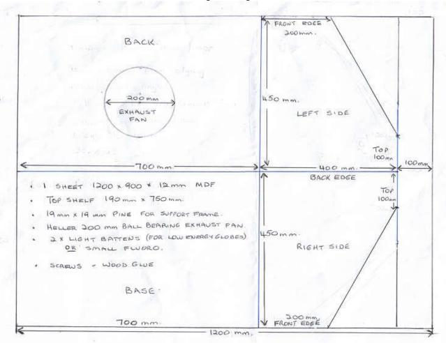
These photos show the basic construction of the cutting box - lengths of 19 mm x 19 mm dressed pine have been used to make the cutting box sturdy without needing to use a thicker MDF. This also cuts down on the overall weight of the box.
