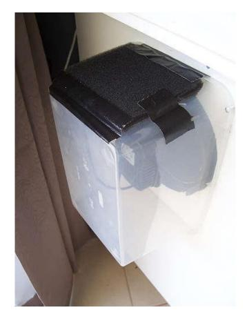
On the inside of the cutting box I used a circle of the same air conditioning filter foam to go between the fan cover and the blades. Some twisty ties hold the foam in place so there is no danger of it being sucked into the blades. The fan cover is easily removed so the filter foam can be washed out
