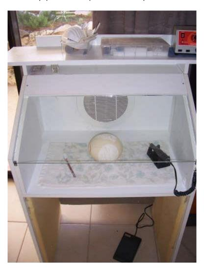
The exhaust fan I used is a Heller Ball Bearing fan which I purchased from Bunnings. Ensure the exhaust fan you choose can be used in the orientation you wish to use. Not all fans will work in a vertical position as they are mainly designed to go in a ceiling. This particular fan also has ball bearings as opposed to sleeve bearings and this is supposed to contribute to the quieter operation of the fan.
