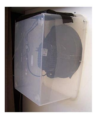
I used two thicknesses of air conditioning filter foam taped over the hole to stop any dust from being pushed out into the room.
