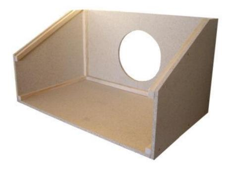
If you put the sides on the outside of the base and the back pieces as I have done here you will need to cut a 50 mm strip off the back piece of wood or you could use it as a backing piece to the top shelf which will sit across the top of the box to stop things falling off the back.
