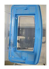
Use a large diamond wheel to cut the opening behind the insect lid—clean up the edges with a craft knife.
