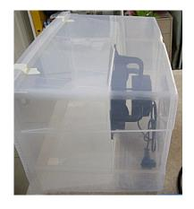
Four lengths of masking tape will be an advantage to hold the two storage boxes together until you get the sides positioned and held in place.
