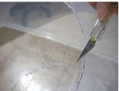
Cut out the circle in the bottom of the storage box - a large diamond wheel like the type used for cutting ostrich eggs in a Dremel or Ozito tool is ideal for this. Clean up the edges using a craft knife.
