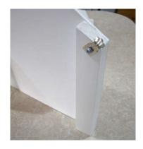
Cut the length of aluminium angle 570 mm long to act as a support for the Perspex across the front. This will be held in place using the mirror supports screwed into the side supports. A bumper screwed onto the front of the upright will stop the aluminium from slipping out from under the mirror support
