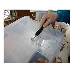
Drill 3 more holes in the lid and then fix in place using nuts and bolts.
